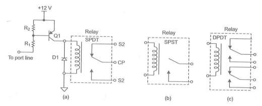
fig 5.11 Interfacing diagram of relay with 8051
