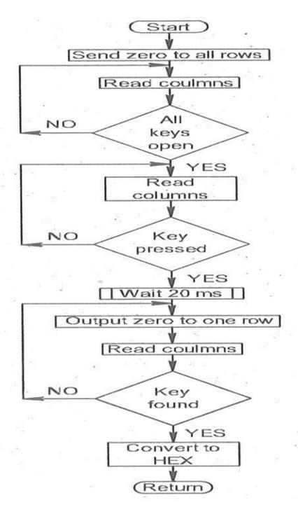
Fig 5.19 flow chart for keyboard scanning subroutine
