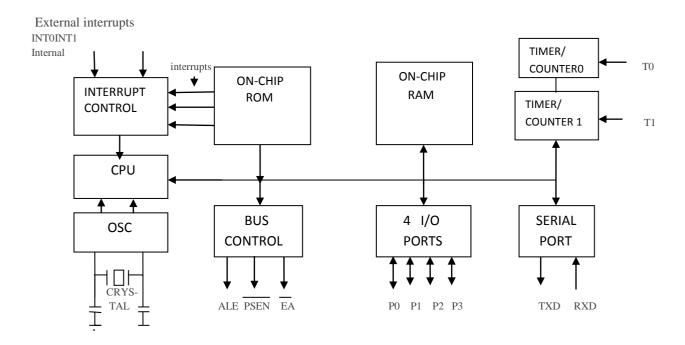
Fig 1.1 Block Diagram of Microcontroller
