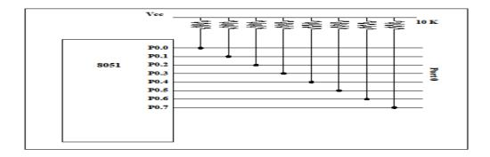
Fig 3.3 Port 0 with Pull-up resistors
