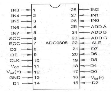
Fig 5.15 pin diagram of ADC 0808
