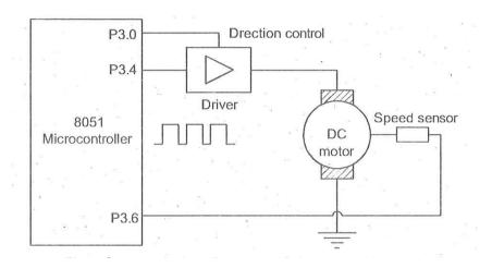
Fig 5.26 Interfacing diagram of DC motor 8051
