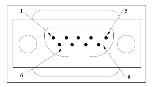
Fig 4.5 DB – 9 9-Pin Connector
