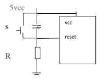
Fig 1.11 Power on reset circuit
