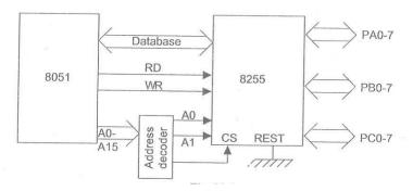
Fig 5.3 (b) Interfacing 8255 with 8051
