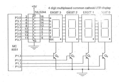
Fig 5.21 7 – Segment LED Display interface with 8051
