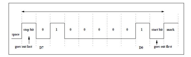
Fig 4.3 Framing ASCII "A" (41H)
