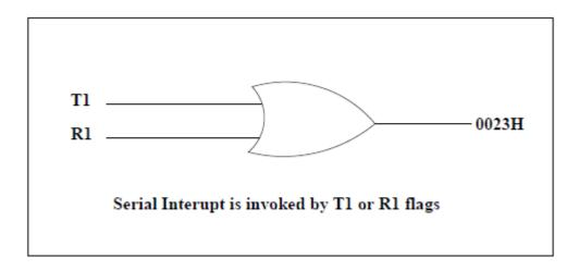
Fig 4.16 Single Interrupt for both TI and RI
