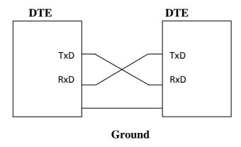
**Fig 4.6 Null Modem Connection**
