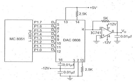
Fig 5.17 Interfacing diagram of DAC with 8051
