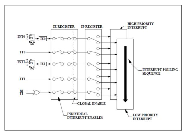
Fig 4.11 Interrupt Structure of 8051 Microcontroller
