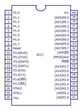
Fig 1.2 Pin Details Of 8051
