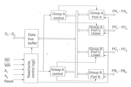
Fig 5.2 Functional block diagram of IC
