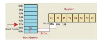
Fig 1.8 Function of Stack Memory
