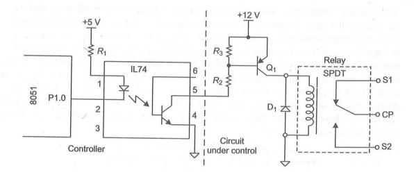
Fig 5.12 Interfacing And Opto Coupler
