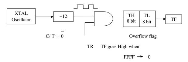
Fig 3.9 Mode 1 Operation:16-bit Timer Mode
