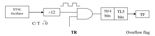
Fig 3.8 Mode 0 Operation: 13-BIT TIMER MODE
