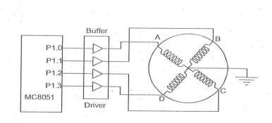
Fig 5.24 Interfacing diagram of stepper motor with 8051
