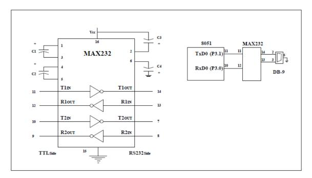
Fig 4.8 (a) Inside MAX 232 (b) Connections to the 8051( Null Modem )
