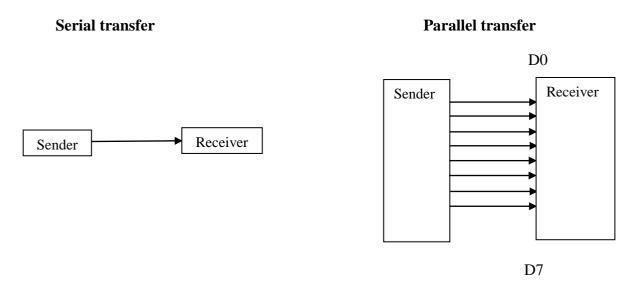
Fig: 4.1 Serial Versus Parallel Data Transfer
