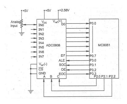
Fig 5.15 (a) Interfacing diagram of ADC 0808
