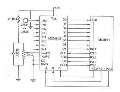
Fig 5.14 Interfacing diagram ADC0808 with 8051
