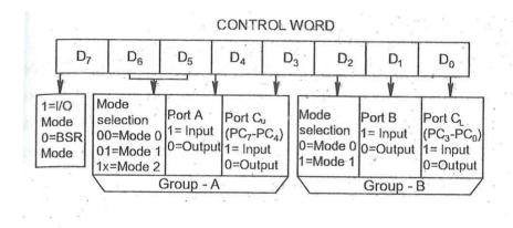
Fig 5.4 Control world format for I/O Mode
