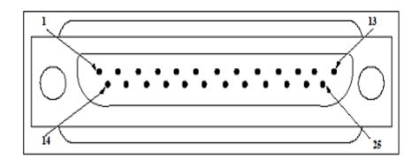
Fig 4.4 RS 232 Connector DB - 25
