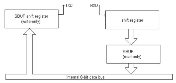
Fig 1.9 Diagram of Serial port
