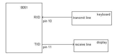
Fig 1.10 Diagram of Serial Communication
