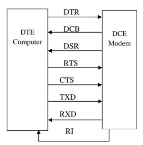
Fig 4.7 Hand Shaking Signals
