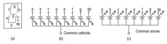
Fig 5.20 (a) Diagram of 7-segment LED (b) diagram of common cathode 7-segment(c)diagram common anode 7-segment
