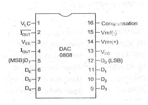
Fig 5.16 pin diagram of DAC 0808
