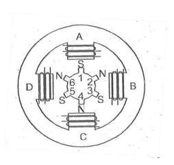
Fig 5.22 Schematic diagram of Stepper motor
